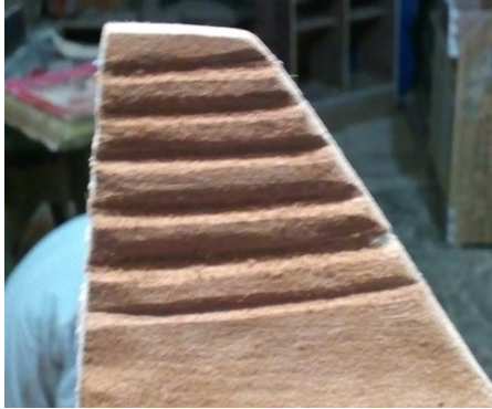
Figure 2: Corrugations of Winglet
